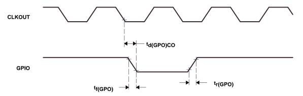
Figure 28. General-Purpose Output Timing
