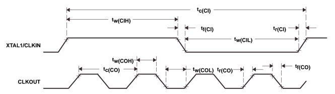
Figure 16. CLKIN-to-CLKOUT Timing with PLL and External Clock in  $\times 4$  Mode
