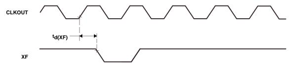
Figure 24. XF Timing
