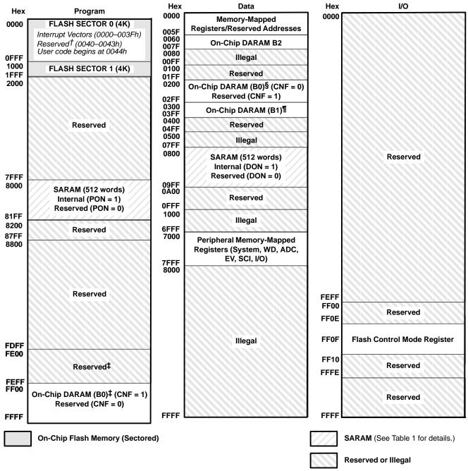
NOTE A: Boot ROM: If the boot ROM is enabled, then addresses 0000-00FF in the program space will be occupied by boot ROM. † Addresses 0040h–0043h in program memory are reserved for code security passwords.
