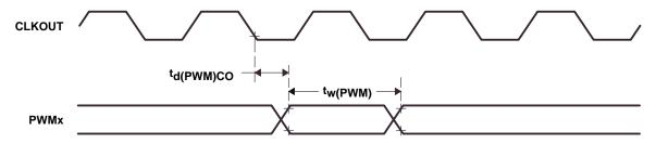
Figure 25. PWM Output Timing
