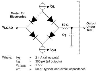
Figure 13. Test Load Circuit
