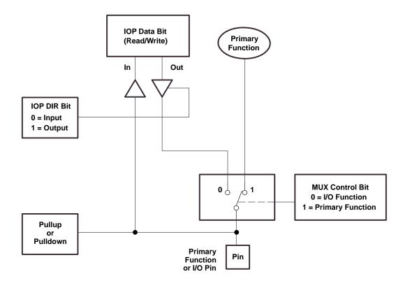
Figure 9. Shared Pin Configuration
