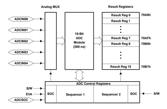
Figure 5. Block Diagram of the 2401A ADC Module
