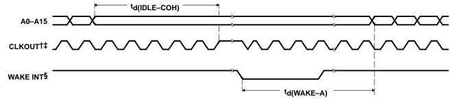
† In 2401A, CLKOUT will not be seen at the pin, only in some modes; it can be enabled in software.
