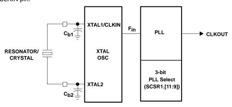
Figure 7. PLL Clock Module Block Diagram
