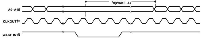
† In 2401A, CLKOUT will not be seen at the pin, only in some modes; it can be enabled in software.
