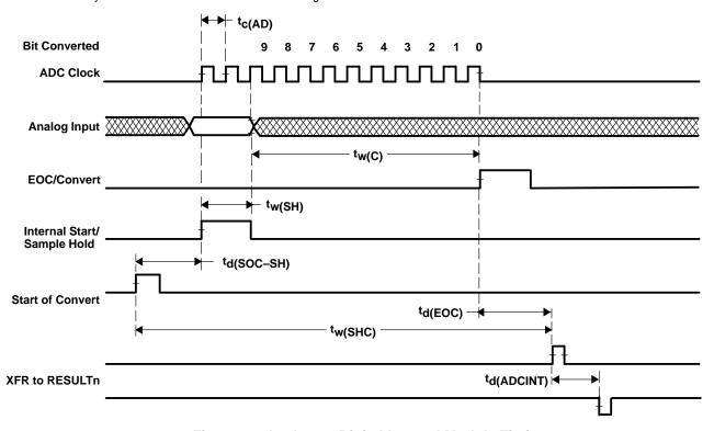
Figure 30. Analog-to-Digital Internal Module Timing
